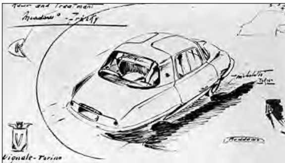
Michelotti's Sketch of the Frisky showing the Gull wing door concept
